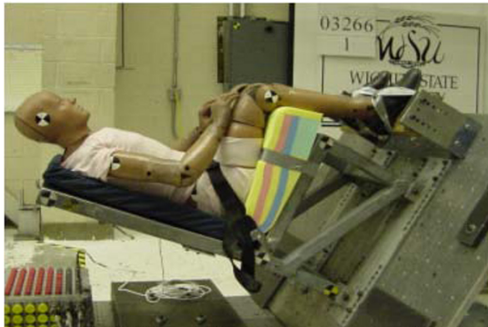
Fig. 5. Full scale sled test for validating the mathematical dynamic model.
